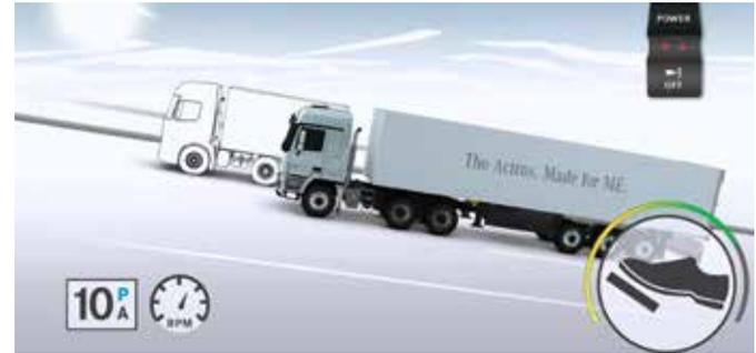
Power mode is activated at the touch of a button, enabling the driver to call upon enhanced power over a short period. This increases the vehicle's agility and allows the driver to mobilize power reserves in specific situations, e.g. on uphill stretches, when joining motorway traffic or when overtaking. Power mode is deactivated automatically after ten minutes and the system returns from a power-focused to a consumption-optimized driving style.
