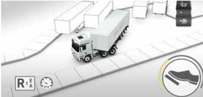
Exact, smooth start-off and precisely metered vehicle motion – the maneuvering mode ensures optimum comfort and safety even in difficult driving scenarios. Sensitive clutch control is guaranteed by providing the full range of the accelerator pedal and engine speeds up to 1,000 rpm. Maneuvering mode can be operated in the first forward gear and the first reverse gear.
