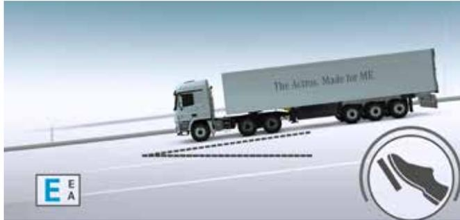
EcoRoll mode supports the driver by keeping the truck rolling without touching the pedals. It is activated at speeds exceeding 55 km/h, when the driver or the cruise control do not accelerate or brake for at least 1 second. Powertrain deceleration is interrupted by automatically setting the transmission to a neutral position. As soon as the brake or accelerator is applied again, the correct gear is selected automatically.
